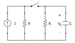
The switch in the figure is **open** for t < 0, **closed** for  $0 \le t < t_1$ , and **open** for  $t \ge t_1$ , where  $t_1 = 3RC$ . Find and plot the voltage  $V_c(t)$ .
