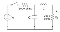
The switch in the figure is **open** at t < 0 and **closed** at  $t \geq 0$ . Find possible values for L and C if the natural response is described by the equation:
