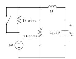
The switch in the figure is **closed** at t < 0 and **open** at  $t \geq 0$ . Find  $V_c(t)$  for  $t \geq 0$ .
