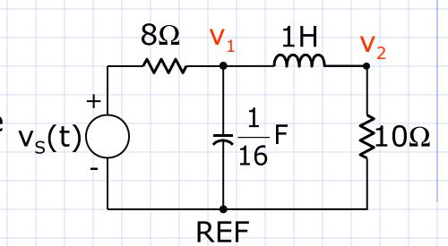
First, write the node equations for the circuit.
