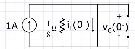
Since the inductor is shorted,  $v_c(0^-) = 0 \text{ V}$  and  $i_L(0^-) = 1 \text{A}$ . Thus,  $v(0^+) = 0 \text{ V}$ .
