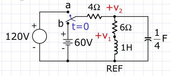
In a previous example, we got the differential equations that describe the voltages  $v_1$  and  $v_2$ . In another example, we derived the initial conditions.
