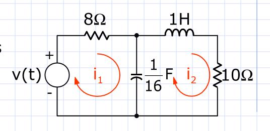
First, write the mesh equations for the circuit.
