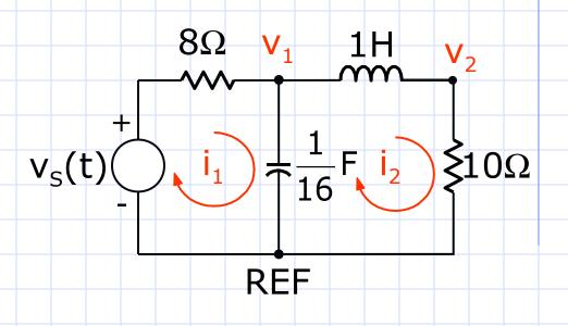
The differential equation for the mesh currents are
