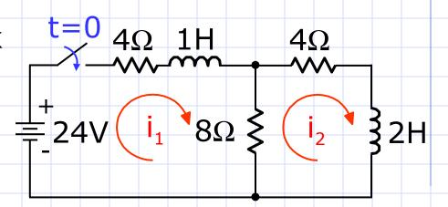
First, get the differential equations that describe currents  $i_1(t)$  and  $i_2$  for  $t \ge 0$ . The mesh equations are
