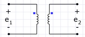
The voltages from the marked terminals to the unmarked terminals have the same polarity.
