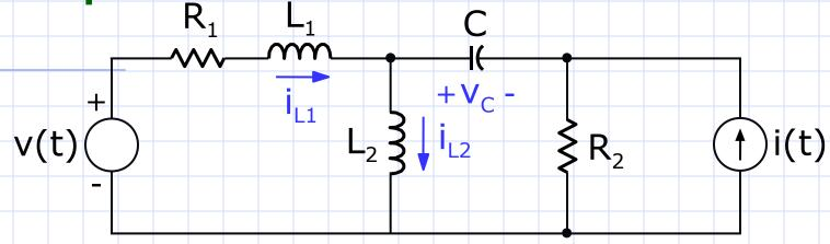
$$i_{L_1}^{\bullet} = \frac{-(R_1 + R_2)}{L_1} i_{L_1} + \frac{R_2}{L_1} i_{L_2} - \frac{v_c}{L_1} + \frac{v(t)}{L_1} + \frac{R_2}{L_1} i(t)$$
