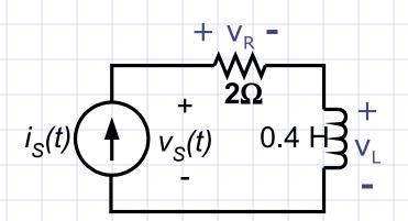
KVL around the loop,  $v_S = v_R + v_L$
