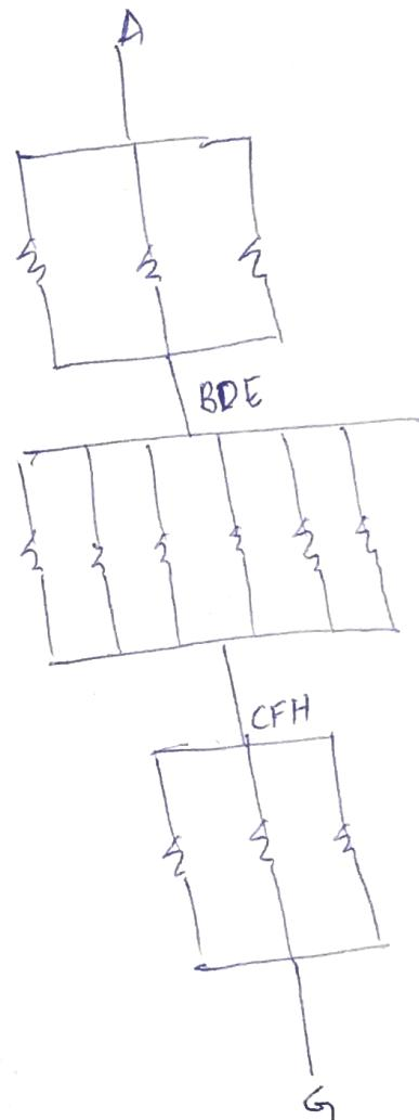
$$\text{Req} = \frac{5}{3}(R \parallel R \parallel R) + (R \parallel R \parallel R \parallel R \parallel R)$$
