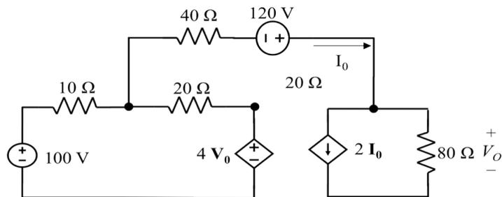
**Figure 9. Using nodal analysis to find the unknown parameters**
