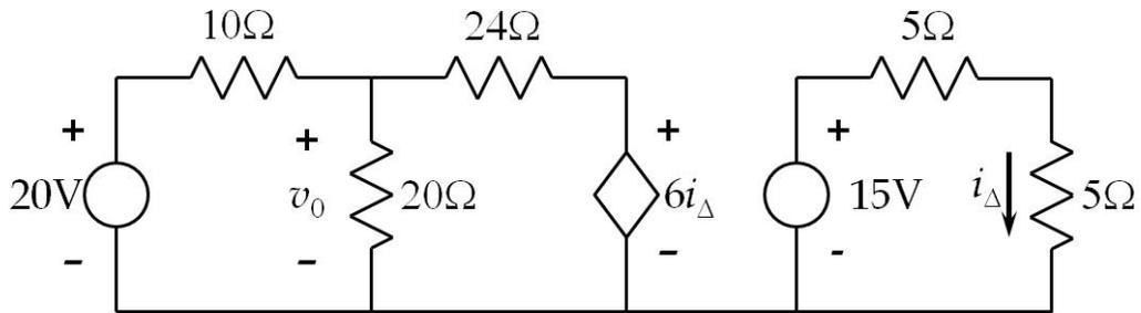
**Figure 8. Using mesh-current method to find  $v_0$**
