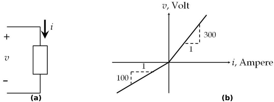
**Figure 1. (a) Device and (b) its voltage-current plot**
