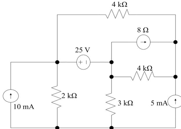
**Figure 4. Using nodal analysis to determine the power generated**
