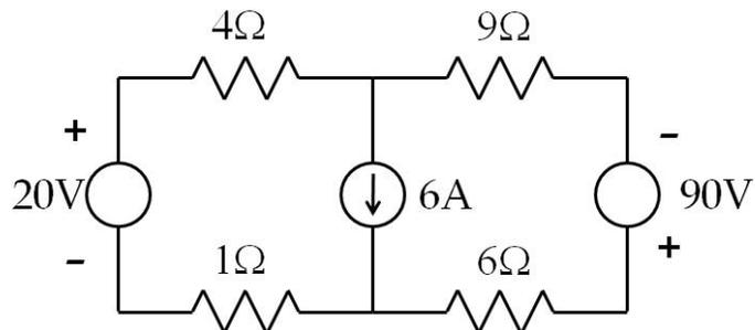
**Figure 7. Using mesh-current method to find unknown power**
