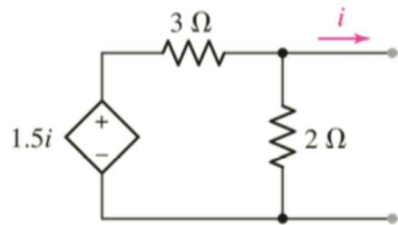
Apply Vtest, the resulting node voltage equation becomes:
