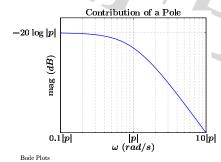
Bode plot is similar to the Bode plot of an RC filter.
