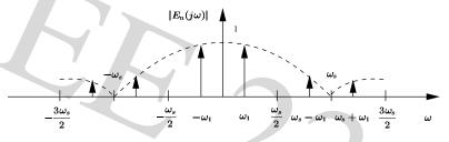
• The frequency response of the zero-order hold determines the magnitude spectrum of the sample and hold output.
