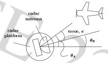
• Since  $\theta_A(t)$  is the angle to the aircraft and  $\theta_R(t)$  is the direction where the antenna is pointing,
