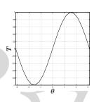
ullet Torque on pendulum mass is  $T = MgL\sin\theta$ . Relationship between T and  $\theta$  is nonlinear.
