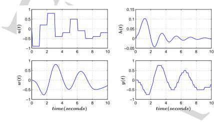
©2003 M.C. Ramos UP EEE Department  $\bullet$  The signal is then sampled at 10 Hz and 3-bit quantized
