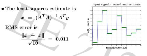
• If we did not filter the input the RMS error would have been 0.035 (due to quantization errors).
